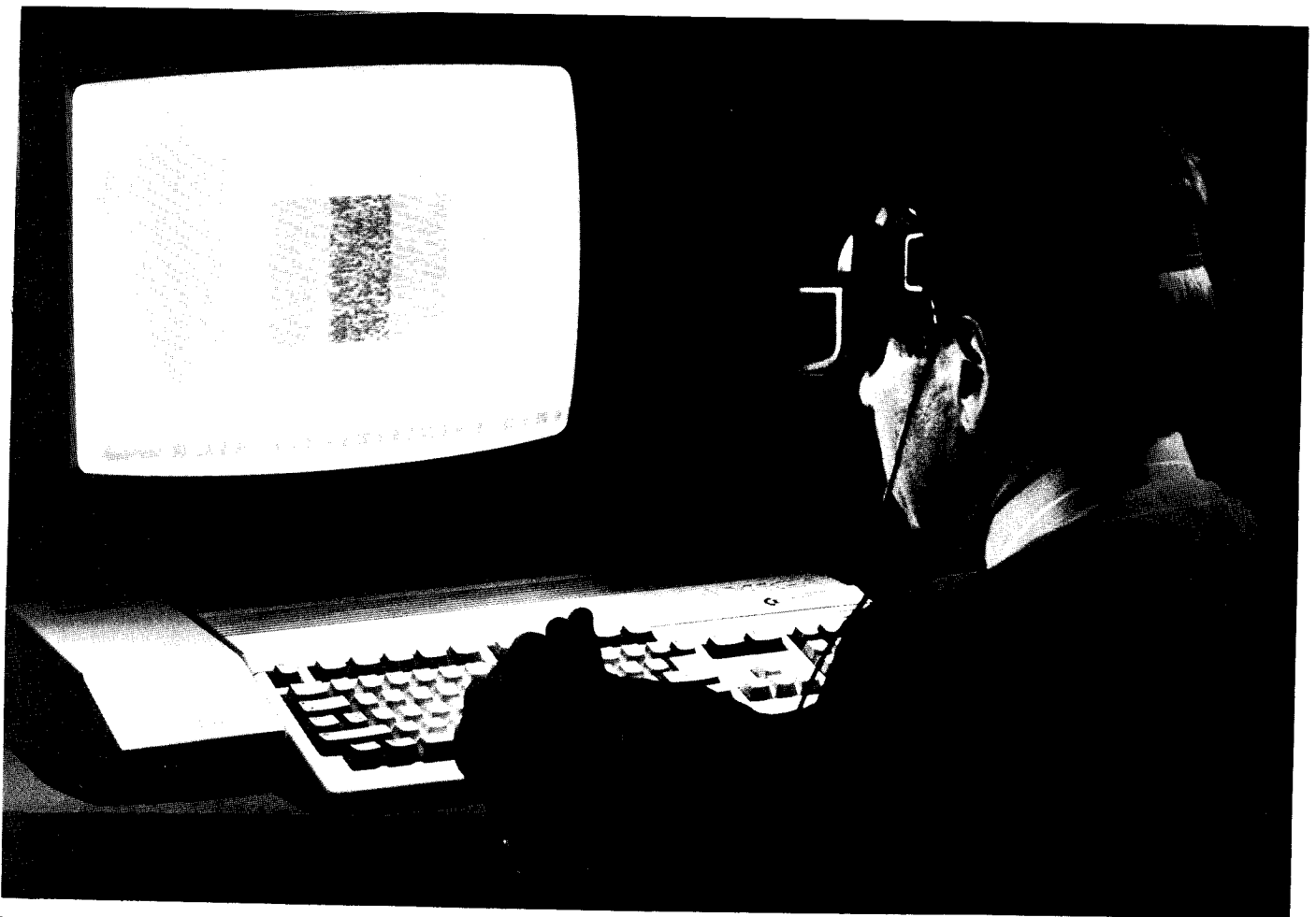
Figure 1 (Feldman et al): Experimental Apparatus: An electronic haploscope. (Computer Orthoptics™ Vergence II LCD System, RC Instruments, Cicero, Indiana) The subject is wearing liquid crystal glasses. The glasses are connected to a dedicated Amiga 2000 HD computer system with interaction hardware and software. The subject views the monitor which presents the dichoptic stimuli (See Figure 2). Various stimulus parameters, as well as the subject's responses, can be manipulated or measured by either joystick or keyboard input.
